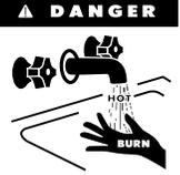
**Water temperature over 125 degrees F. can cause severe burns instantly, or death from scalds. Children, disabled, and elderly are at highest risk of being scalded. See instruction manual before setting temperature at water heater. Feel water before bathing or showering! Temperature limiting valves are available.**
